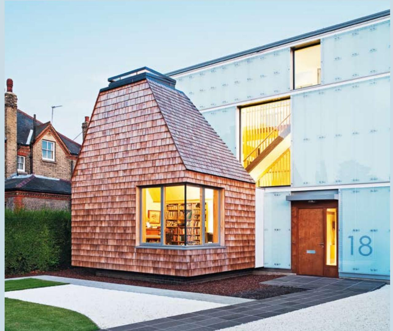
*left Made from cross-laminated timber panels and part clad in a shimmering glass screen, the modern geometric structure contrasts with the classic Victorian terraced houses in the same street*
